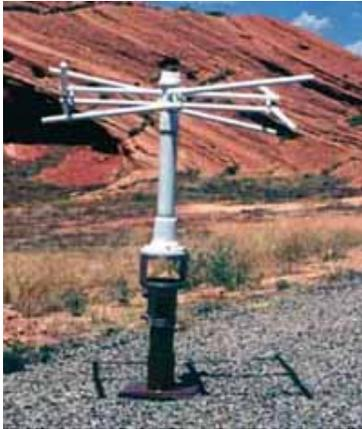
The single element dBs 100 VDB antenna is an elliptically polarized, VHF data broadcast antenna. It exhibits an omnidirectional azimuth pattern and a shaped vertical pattern, which is similar to a dipole.
