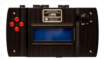
**SCREEN SPECS**: 3.125" screen, LCD 4 X 20 character display, blue display with white LED
