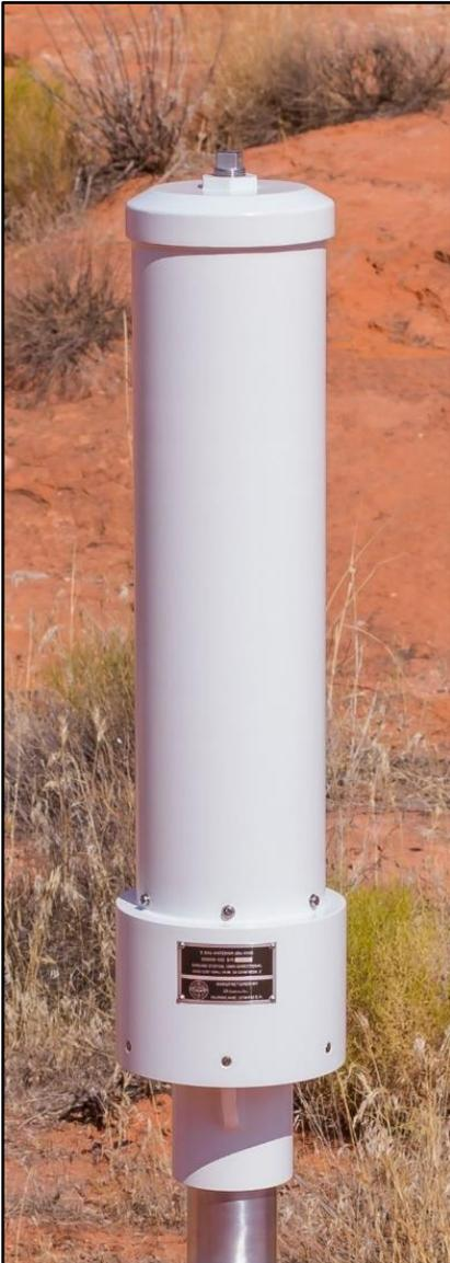
The dBs 5000 is an omni-directional broadband, 10 element, high performance, collinear dipole phased array designed specifically for use as a 5 GHz ground uplink antenna. It exhibits low side lobe levels and negative angle radiation (minimizes multipath). The above-the-horizon null-filled pattern minimizes the radiated cone of silence. The antenna handles input power to 10 watts and operates over its entire frequency range with an input VSWR at 50  $\Omega$  of less than 2.0:1.
