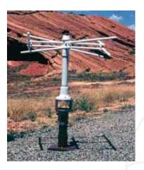
The single element dBs 100 VDB antenna is an elliptically polarized, VHF data broadcast (VDB) antenna. It exhibits an omni-directional azimuth pattern and a shaped vertical pattern, which is similar to a dipole.
